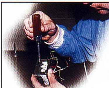
A 'Minor' Screwdriver tightening fasteners on delicate electronic equipment.
